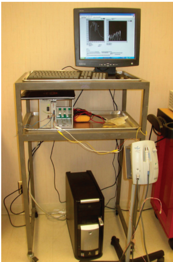
Figure 4. Thermocautery tip coupled to thermocouple and monitoring equipment.
