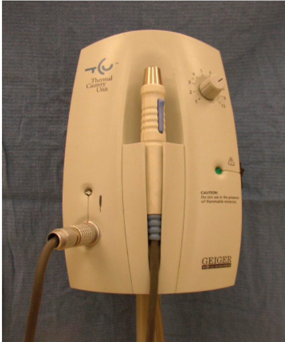
Figure 1. Tunable, electrically powered thermocautery unit (Geiger model 150).
